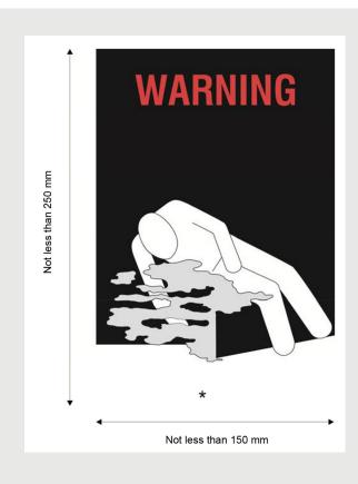
The \* shall be replaced with the words CARBON DIOXIDE SOLID or DRY ICE and remain in place until the vehicle is completely unloaded and any concentration of  ${\bf C0}_2$  dispersed.
