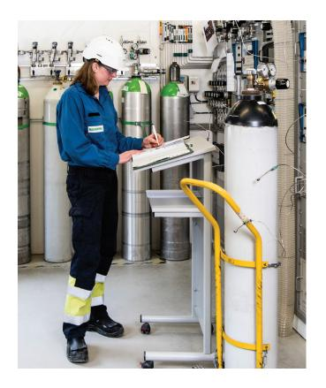
AccuDew® is a series of calibration gases developed to reduce the uncertainty when measuring moisture in gas streams.
